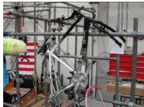
The frames were fastened securely to a very solid scaffolding arrangement
