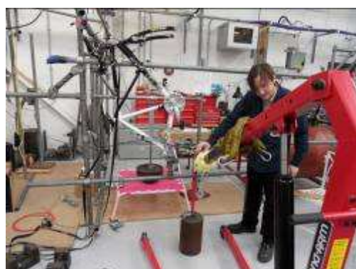
The weight being lowered onto the wheel
