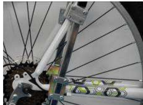
It is necessary to ensure the clamps are positioned correctly for maximum support to prevent rotation
