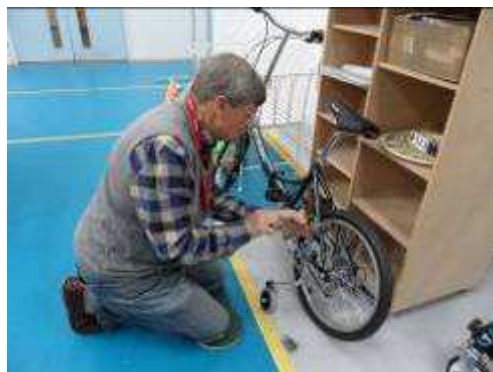
Fitting Standard Adjustabilisers to a folding style city bike.
